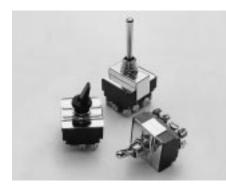
The I-Series toggle switches are heavyduty, four pole switches with a slowmake, slow-break contact mechanism. These switches are available in a wide range of terminations, circuits and bushing/toggle configurations.
